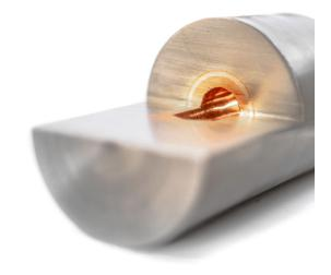
The Dycobond<sup>®</sup> process revolutionizes the internal mold cooling by inserting a thick, multilayer lining into the cooling channel made in a single working step directly during the hardening process.
